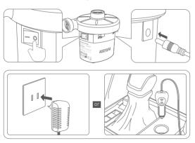
Choose the appropriate nozzle and inflation/deflation port to use based on the type of item being inflated or deflated. Then, securely insert the nozzle into the inflatable and press the "—" Switch. The air pump will start work.
