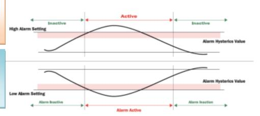
When an alarm condition occurs, **HI-ALARM** and **LO-ALARM** icons will appear on the display along with a beeping sound to alert user. The beeping sound will stay ON until the unit gets back in range. **Press any key ONCE to stop the beeping sound.**
