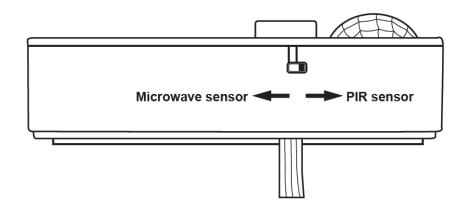
Switch between Microwave Sensor and PIR Sensor.
