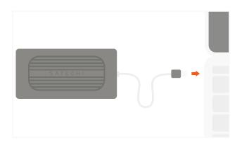
Use the HDMI port to output 4K HDMI to an external monitor or display – up to 60Hz.
