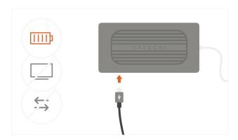
4 Use USB-A data ports to connect USB devices – 2 x USB 3.2 data up to 10 Gbps each and 1 x USB 2.0. Does not support charging or CD readers, including Apple SuperDrive
