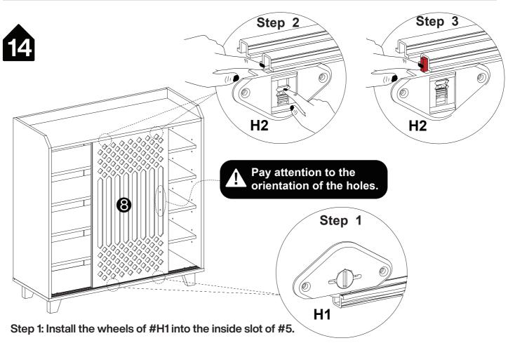
Step 2: Press the limit spring of #H2 down, and then align the corresponding stopper with the inner slot of #1.
