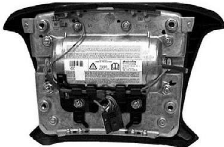
Fig. 4: Identifying Driver'S Front Airbag Courtesy of BMW OF NORTH AMERICA, INC.
