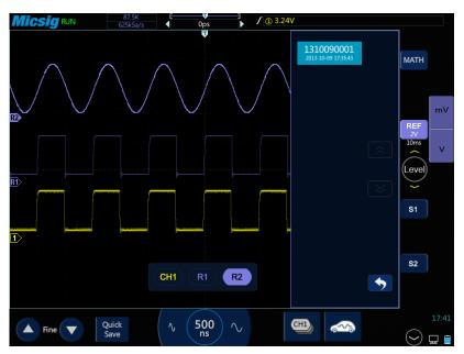
Figure 9-6 Restore Reference Waveform
