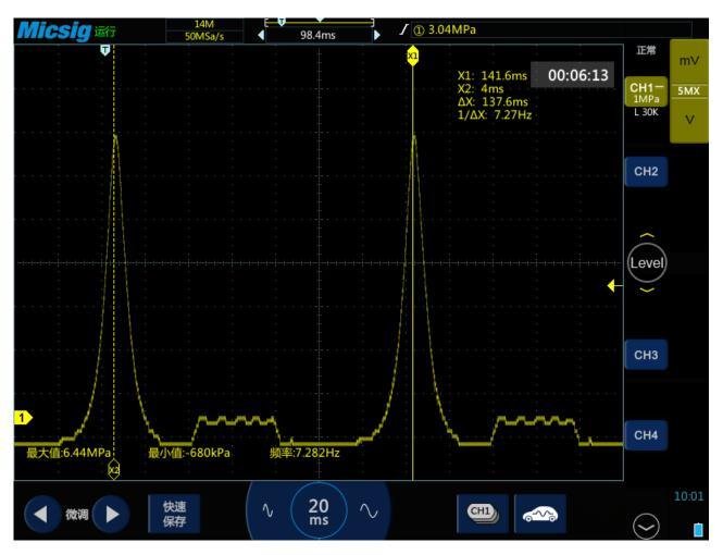
Figure 3-57 Mazda 6 Cylinder internal pressure measurement
