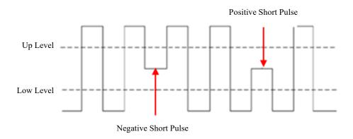
Figure 6-23 Runt Trigger
