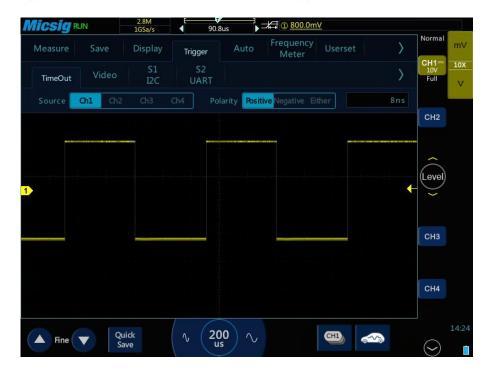
Figure 6-28 Time-out Trigger
