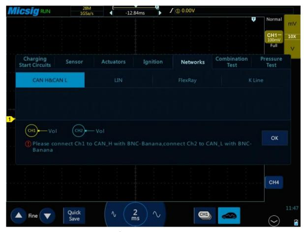
Figure 3-45 CAN BUS Test
