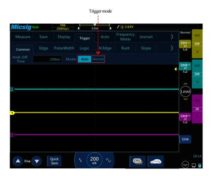
Figure 6-5 Oscilloscope Trigger Mode Setting
