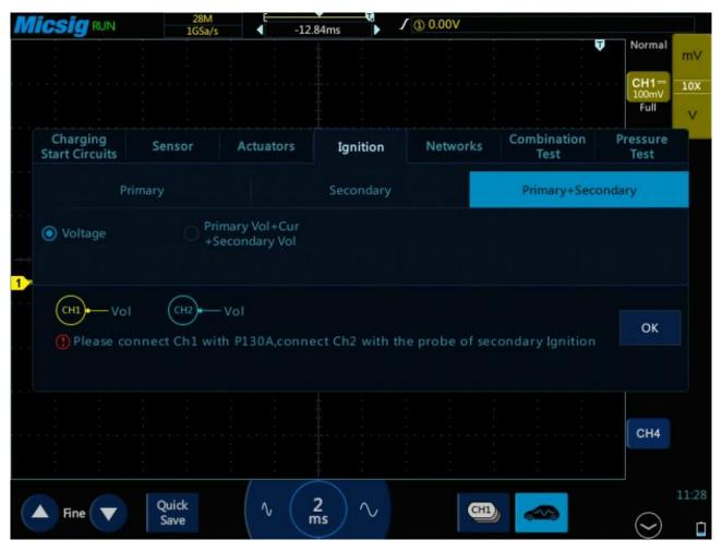
Figure 3-43: Primary + Scondary ignition test
