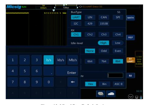
Figure 13-5 Baud Rate Default Setting
