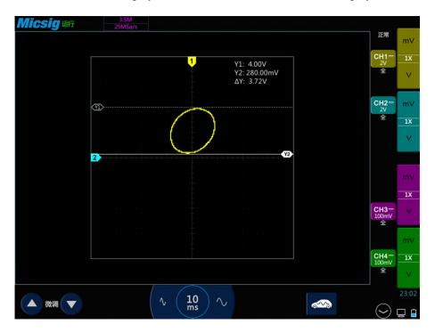
Figure 7-10 In XY Mode, Cursor Measurement
