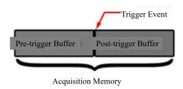
Figure 6-6 Conceptual Demonstration of Acquisition Memory
