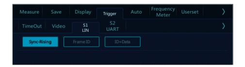
Figure 13-10 LIN Trigger Mode Configuration Menu
