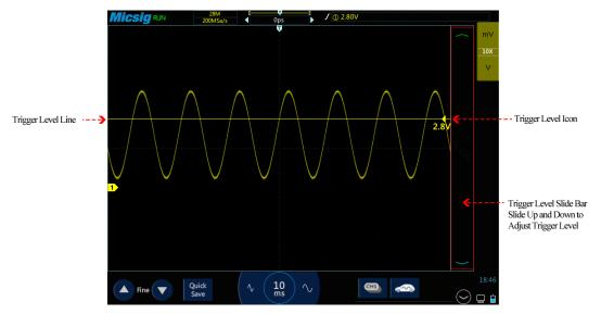
Figure 6-8 Trigger Level
