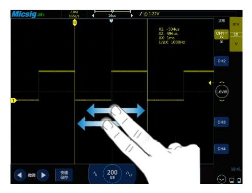
Figure 7-9 Cursor Measurement Pulse Width
