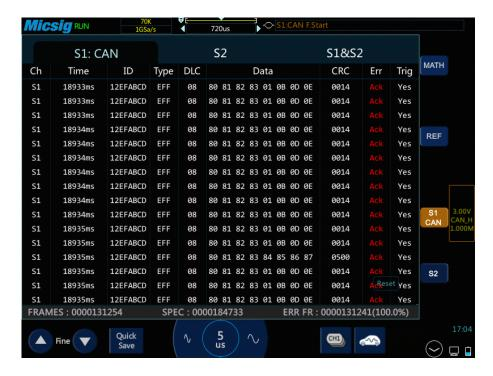
Figure 13-17 CAN Text Interface
