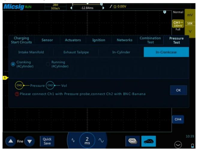
Figure 3-58 Crankcase Pressure and Voltage test
