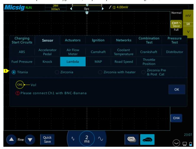
Figure 3-20 Lambda (oxygen sensor) test
