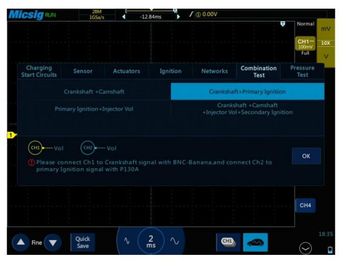
Figure 3-51 Crankshaft + Primary ignition test
