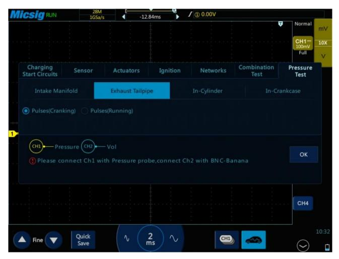
Figure 3-55 Exhaust Tailpipe Test
