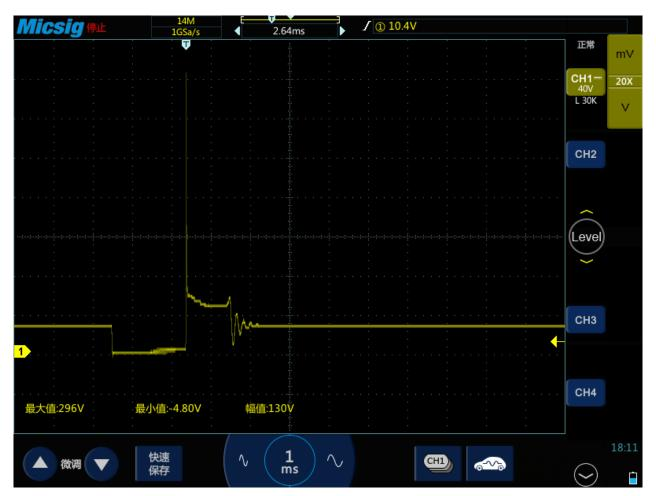
Figure 3-41 Primary ignition actual test
