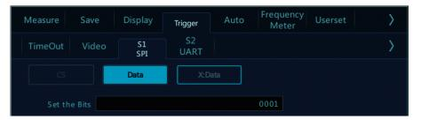
Figure 13-19 SPI Trigger Mode Configuration Menu
