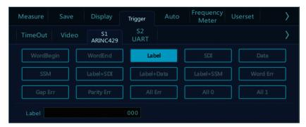
Figure 13-27 ARINC429 Trigger Mode Configuration Menu
