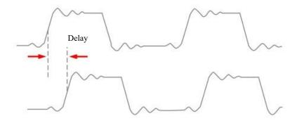
Figure 7-4 Delay Measurement Schematics
