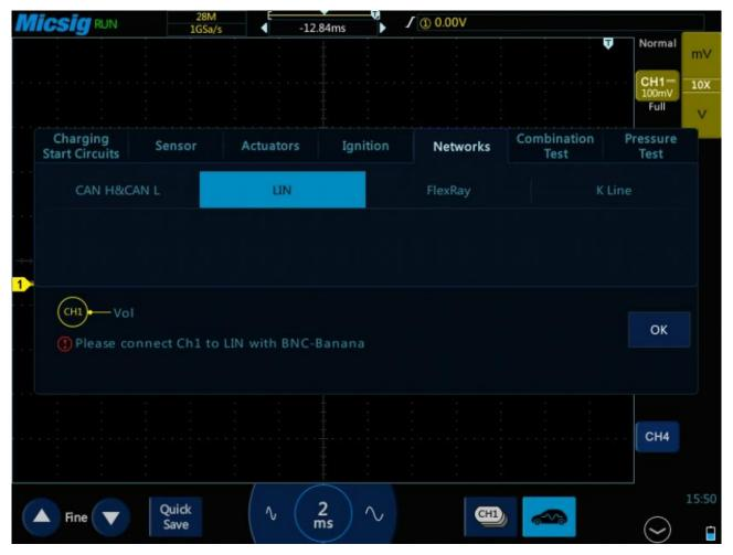
Figure 3-46 Lin bus test
