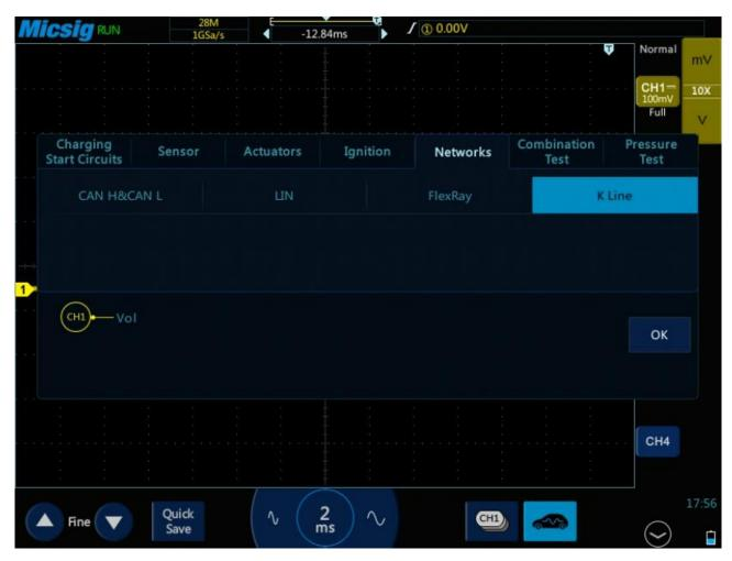
Figure 3-49 K line test
