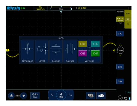
Figure 5-6 vertical position adjustment of waveform
