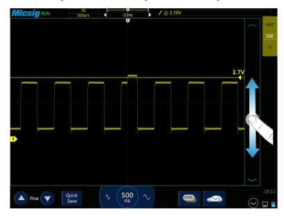
Figure 6-4 Abnormal Signal Captured by Setting Trigger Level
