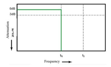
Figure 11-2 Theoretical Brick-Wall Frequency Response
