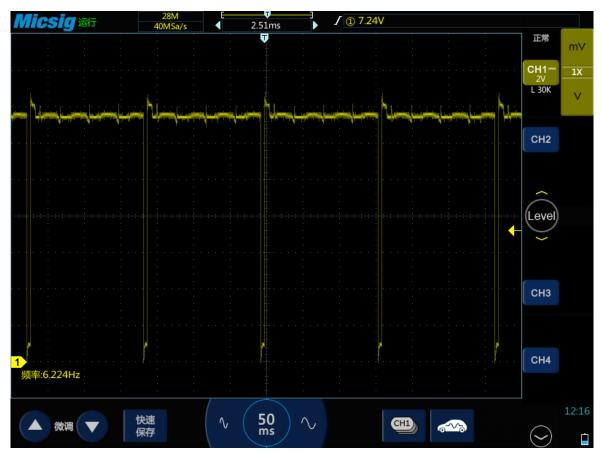
Figure 3-27 Audi A6 Carbon canister solenoid valve signal
