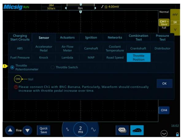
Figure 3-24 Throttle Position Sensor test
