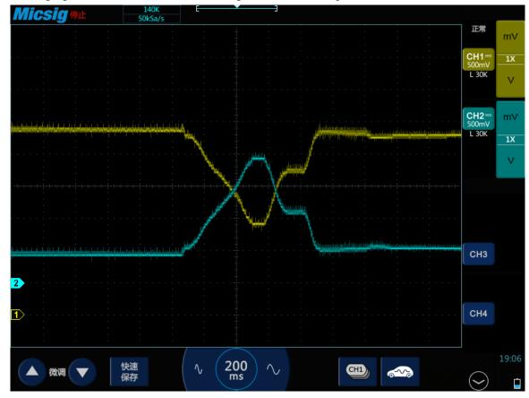
Figure 3-25 Throttle Position Sensor Diagram
