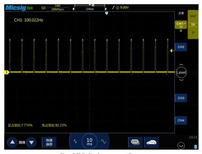
Figure 3-38 Cooling fan measurement diagram
