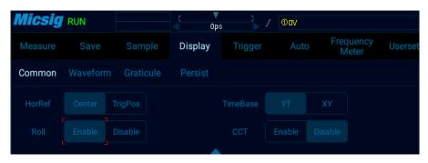
Figure 4-7 Roll Mode On/Off
