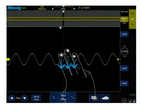
Figure 4-12 Open Zoom Function by Three Fingers Sliding Down
