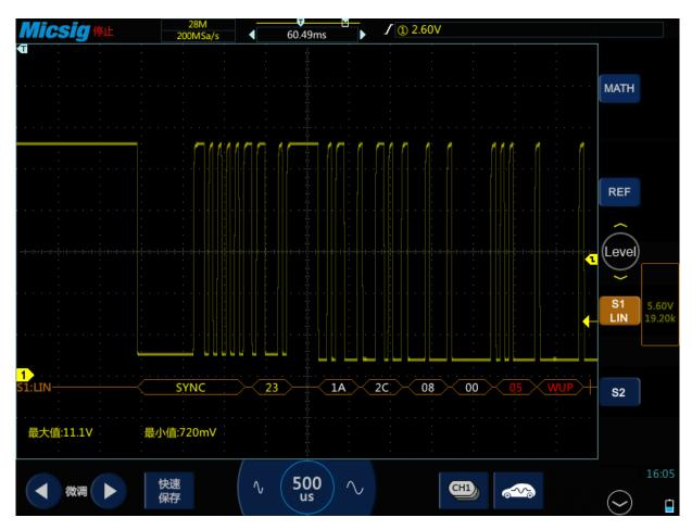
Figure 3-47 Audi A6 LIN bus measurement
