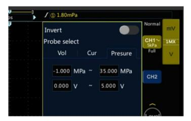
Figure 5-16 Pressure Probe
