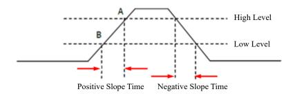
Figure 6-25 Positive/Negative Slope Time
