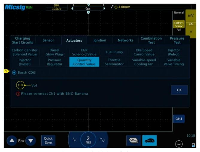
Figure 3-35 Quantity (Flow) control valve test
