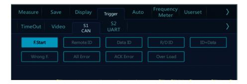
Figure 13-15 CAN Trigger Mode Configuration Menu
