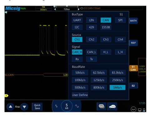
Figure 13-14 CAN Bus Configuration Menu
