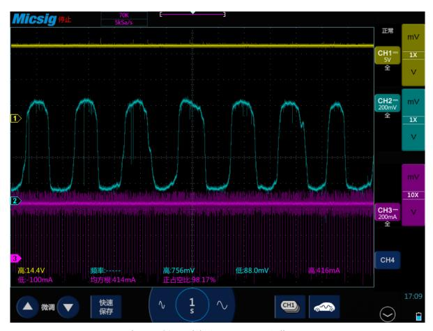
Figure 3-21 Lambda (Oxygen Sensor) diagram
