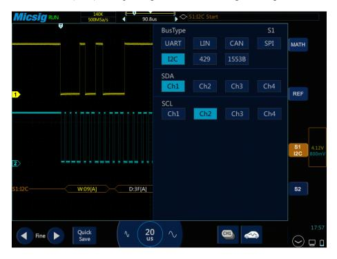
Figure 13-22 I2C Bus Configuration Menu
