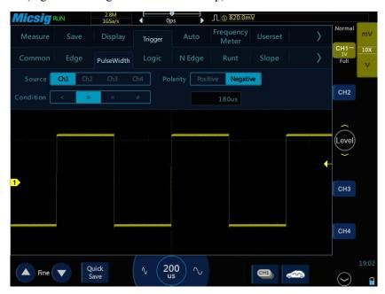
Figure 6-14 Negative Polarity Pulse Level Flip
