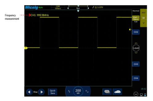
Figure 7-6 Frequency Meter Measurement
