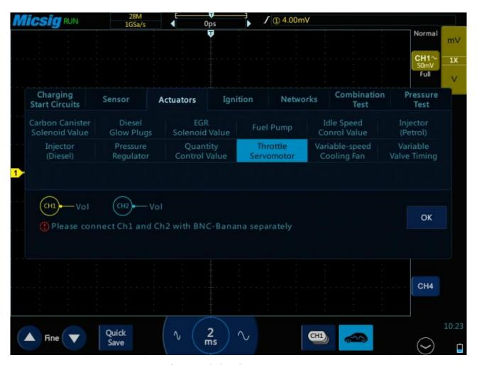
Figure 3-36 Throttle servo motor test
