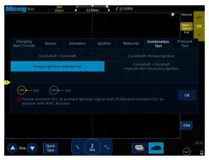
Figure 3-52 Primary ignition + Injector voltage
