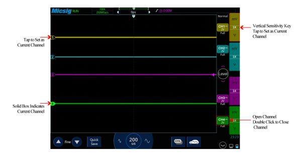
Figure 5-4 Channel Open, Close and Switching
