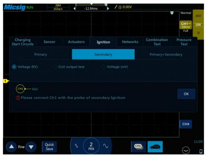
Figure 3-42 Secondary ignition test
