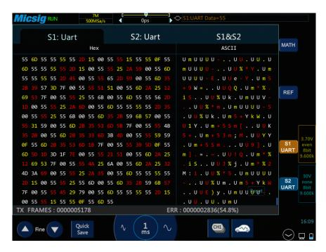
Figure 13-2 Bus Decode Text Mode
