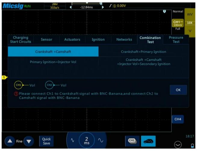
Figure 3-50 Crankshaft + Camshaft Combination Test
