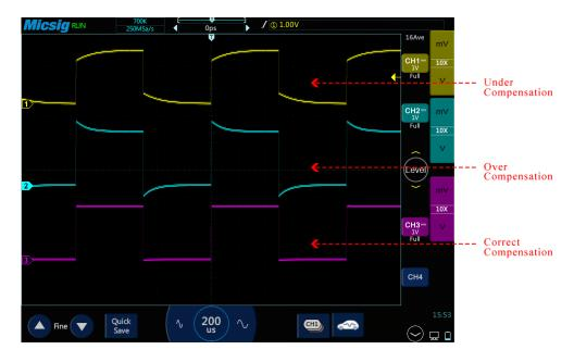
Figure 2-13 Probe Compensation
