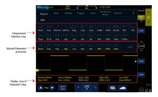
Figure 7-1 Automatic Measurement Menu
