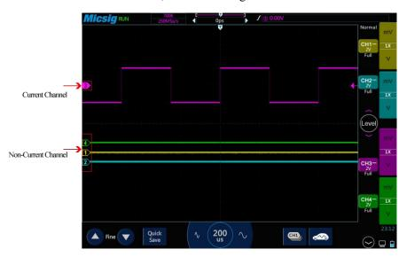
Figure 5-2 Current Channel and Non-Current Channel
