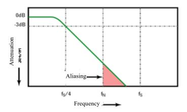
Figure 11-3 Sampling Rate and Oscilloscope Bandwidth
