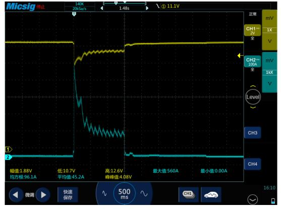
Figure 3-7 Starting voltage and current
