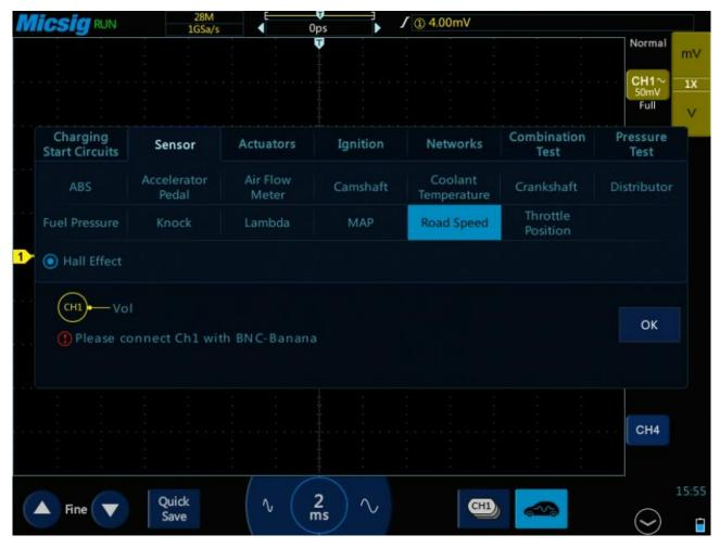
Figure 3-23 Vehicle speed sensor test
