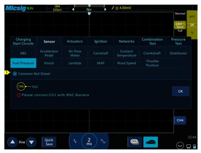
Figure 3-18 Fuel Pressure Sensor Test
