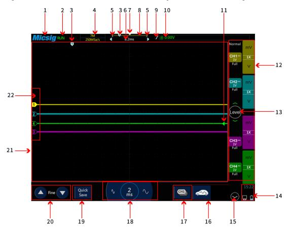
Figure 2-4 Oscilloscope Interface Display
