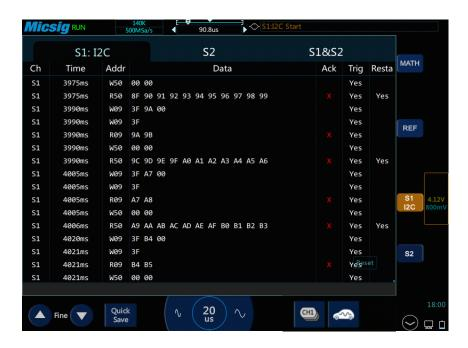
Figure 13-25 I2C Text Interface
