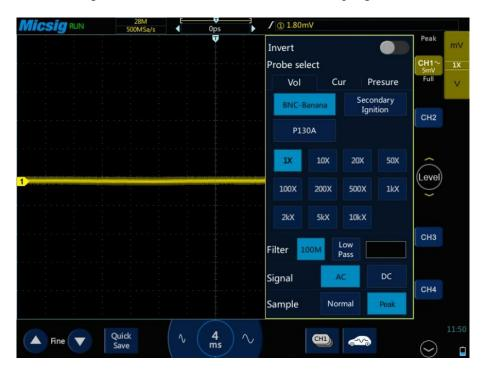
Figure 11-5 Sine Wave with Burr, Peak Sampling Mode
