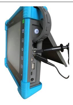
Figure 2-12 Probe Connection
