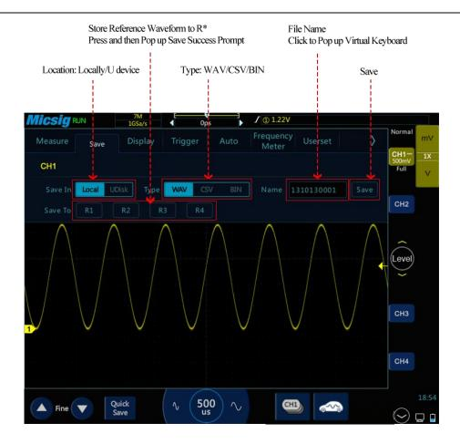
Figure 8-3 Save CH1 Reference Waveform Interface
