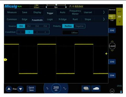
Figure 6-13 Pulse Width Trigger Setting Menu
