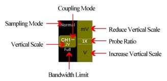
Figure 5-3 Channel Display Interface
