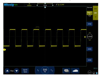
Figure 6-3 Abnormal Signal in Periodic Signals
