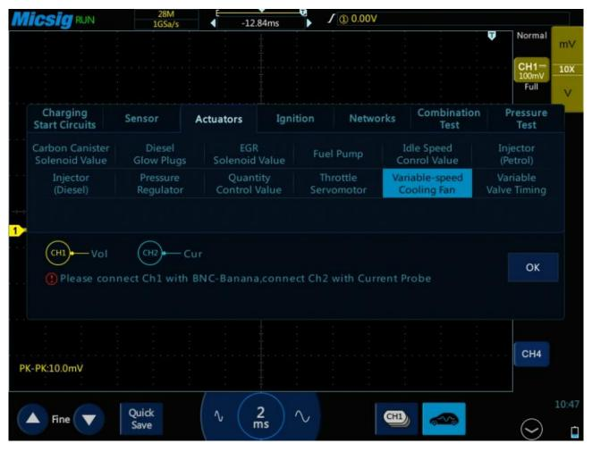
Figure 3-37 Variable-speed Cooling fan test
