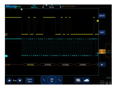
Figure 13-24 I<sup>2</sup>C Graphic Interface
