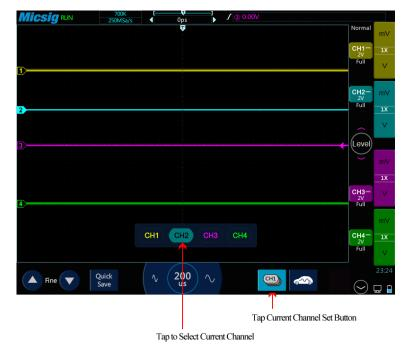
Figure 5-5 Using the Current Channel Selection Button
