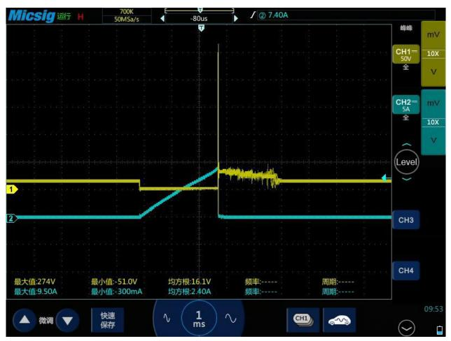
Figure 3-44 BMW 5 Series N20 Primary + Secondary ignition signal
