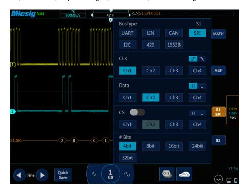
Figure 13-18 SPI Bus Configuration Menu
