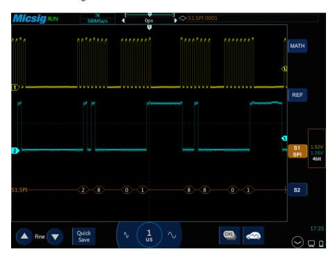
Figure 13-20 SPI Graphic Interface
