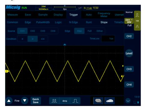
Figure 6-26 Slope Trigger Setting Menu
