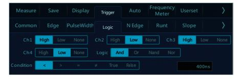
Figure 6-20 Logic Trigger Setting Menu
