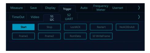
Figure 13-23 I<sup>2</sup>C Trigger Mode Configuration Menu
