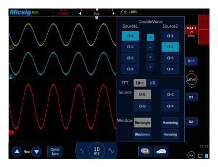
Figure 9-1 MATH Channel Waveform
