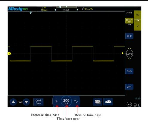
Figure 4-3 Adjust the Horizontal Time Base
