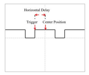
Figure 6-7 Horizontal Delay
