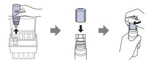
**Note:** Do not leave the ink bottle inserted; otherwise the bottle may be damaged or ink may leak.
