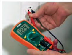
Displays AC Voltage of an outlet receptacle
