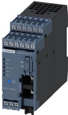
basic device SIMOCODE pro V PN, Ethernet/PROFINET IO, PN system redundancy, OPC UA server, web server, transfer rate 100 Mbps, 2 x bus connection via RJ45, 4 I/3 O freely configurable, Us: 24 V DC, input for thermistor connection monostable relay outputs, expandable by expansion modules
