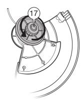
**NOTE:** The Gearbox shaft is a reverse thread. Counterclockwise to tighten, clockwise to loosen.
