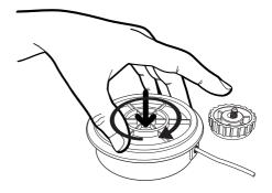
To rectify an incorrectly wound line, fold the line in half, making sure one end is slightly longer than the other. At the fold, hook this onto the inner eyelet. Ensure that both lines are now separated into each section as you tightly wind it round following the indication marker on the top, which is marked 'wind cord'.
