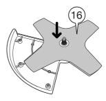
Next, place the Brush Cutter Locking Plate (19) over the drive shaft.
