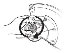
To access the Spool thread, gently push the cover down and twist clockwise to unlock. Carefully lift out the Spool carrier from the case and withdraw the Spool from the eyelets either side. Wipe clean if necessary using a damp cloth. Upon removal, you will notice a spring beneath the carrier
