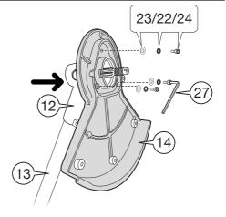
To attach the Plastic Trimmer Guard (15) to the Inner Mounting Plate (14), place the Guard on top an align the 4 holes. Insert 4 x Large Hex Bolts (25) along with the remaining Washers (23) and Spring Washers (22). Securely tighten using the Hex Key (27) supplied.
