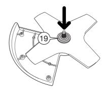
Secure all plates together using the Hex Nut (21) supplied. Tighten using the Maintenance Tool (28). Finally, insert the Split Pin (26) into the small hole of the drive shaft and bend around the Nut.
