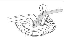
Position the Auxiliary Handle (1) to the Main Unit Pole (5) between the 2 foam grips or where the appropriate po sition is to obtain the best balance. Using the hinged opening, close and secure the Auxiliary Handle (1) using the Auxiliary Handle Locking Screw (2) as shown. Turn clockwise to tighten.
