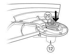
With the Coupling Plate (20) in position, place the Spool Assembly (17) over the drive shaft and turn counter-clockwise to secure.
