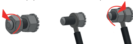
Figure 4. Connecting the unit to an electrical equalizing system.
