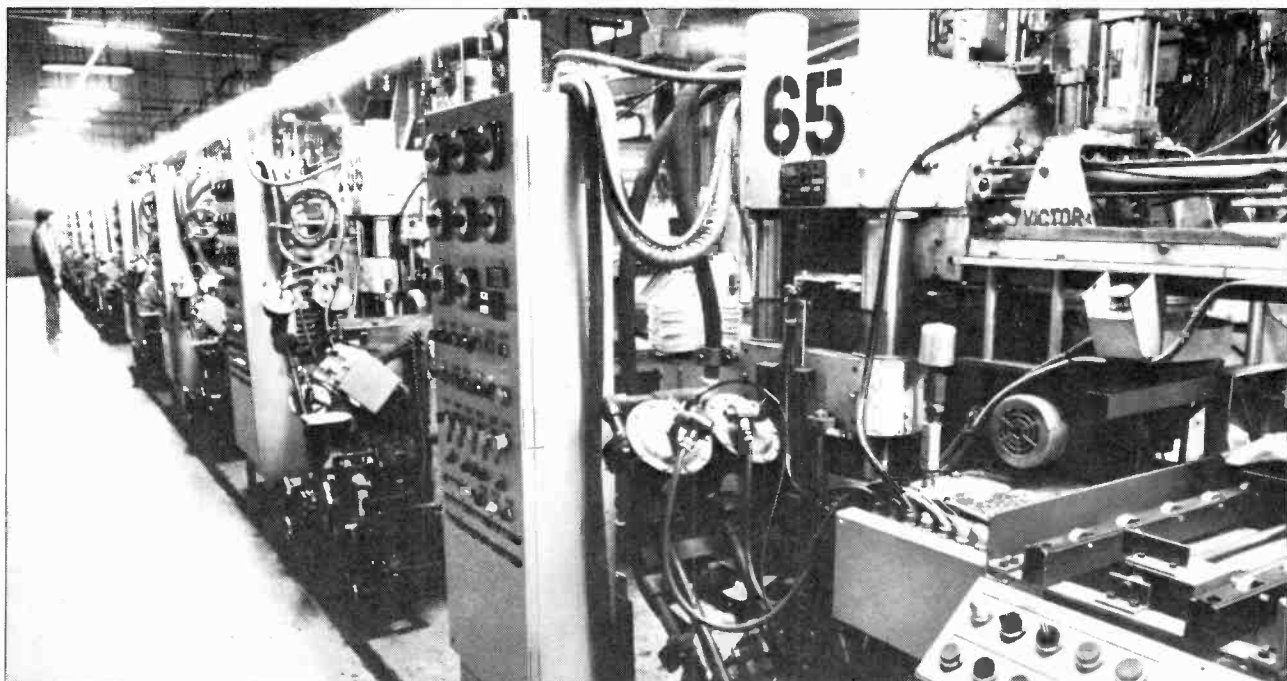
Plant for computer controlled record pressing
