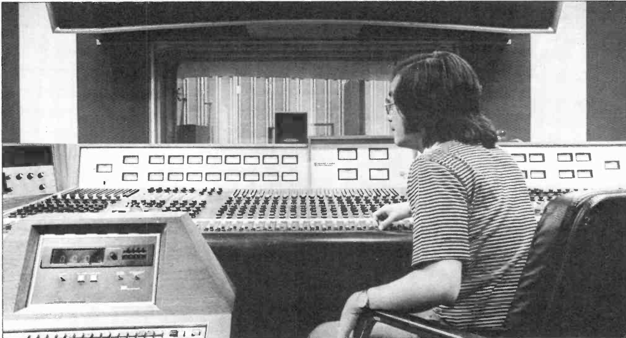
32 channel Mixing Console
