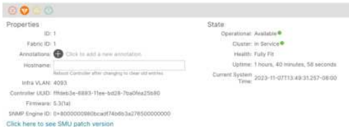
Figure 2: Infra VLAN and Fabric ID of the Cisco APIC
