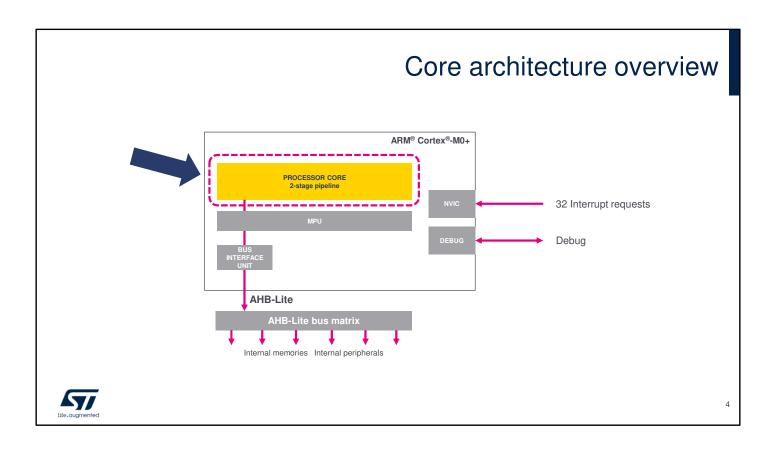
The Cortex®-M0+ core delivers more performance than the Cortex®-M0 core thanks to the 2-stage instruction pipeline. Let's start our description of the CPU by the processor core in charge of fetching and executing instructions.
