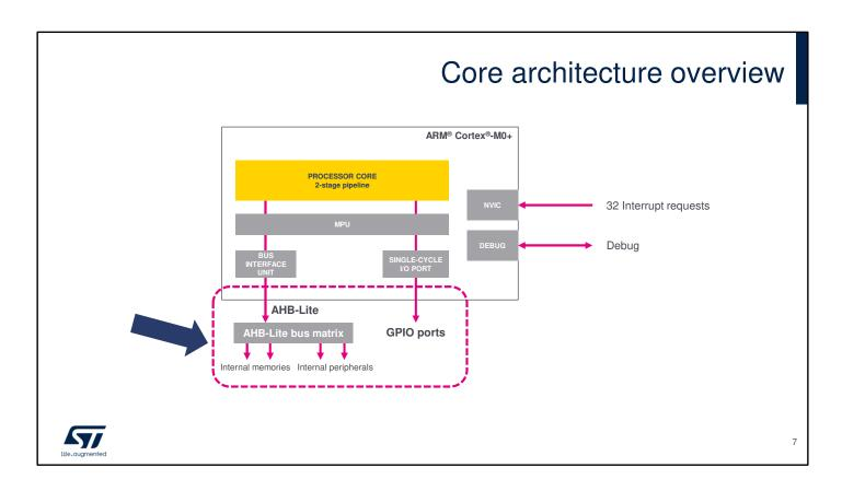
The Cortex®-M0+ has neither an embedded cache nor internal RAM. Consequently, any instruction fetch transaction is steered to the AHB-Lite interface and any data access is steered either to the AHB-Lite interface or the Single-cycle I/O port.
