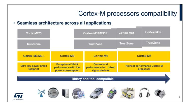
STM32U0 microcontrollers integrate an ARM® Cortex®-M0+ core in order to benefit from the incomparable performance per milliwatt ratio.
