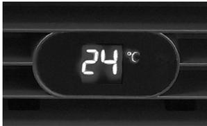
Outlet temperature LCD display
