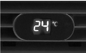
Once the air conditioner is connected to one of the power supplies, the LCD display screen at the front of the air conditioner will show the **Outlet Temperature** in °C.
