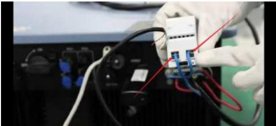
2. Connect one end of the communication cable to the meter. (PIN 4,5 of the communication cable to PIN 5, 6 port of the meter).
