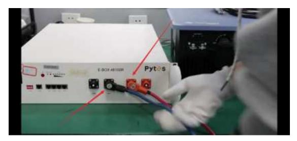
3. Connect the opposite ends of the positive and negative power cables to the corresponding positive and negative terminals of the inverter as shown in the following picture.
