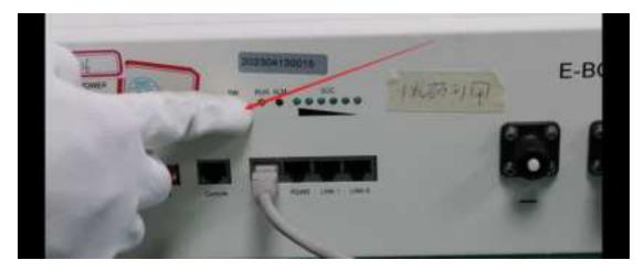
3. Ensure that the RUN light is flashing.
