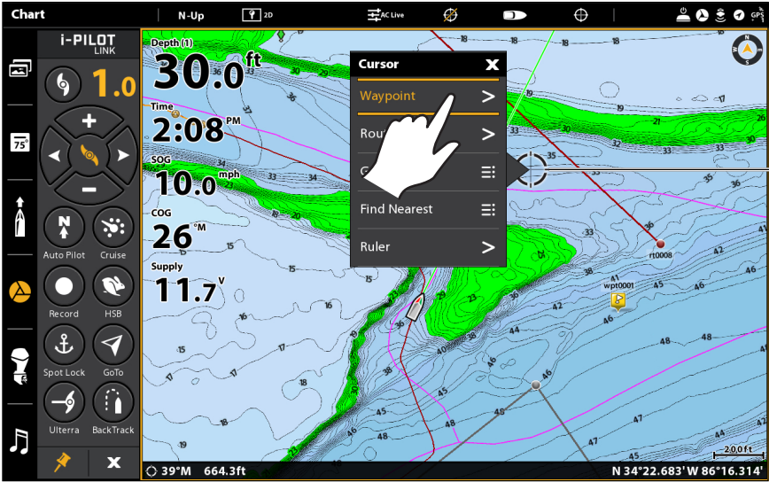
Using the Touch Screen to Mark a Waypoint at the Cursor Position
