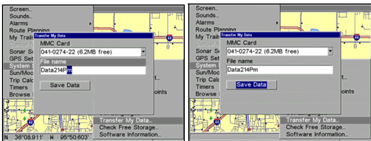
From left to right, these figures show the sequence for naming and saving a GPS Data File from the unit's memory to an MMC.
