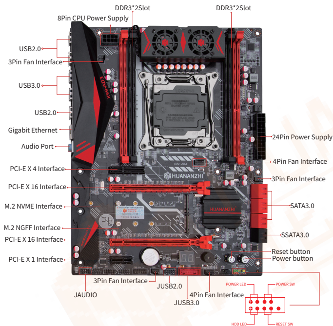
1-1 X99-AD3 V3.0 Motherboard Illustration
