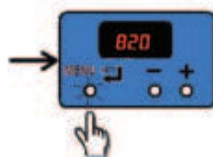
Figure 61. Verify value of 820 rpm
