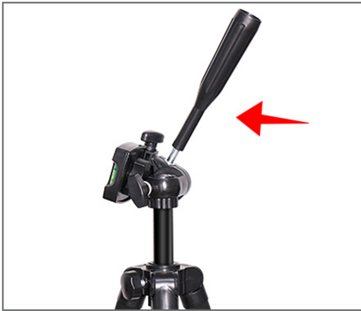
8. Vertical Shooting: Rotate the handle counter-clockwise and tilt the Pan head, allow maximum 90° for vertical use. Clockwise rotate the handle to lock.
