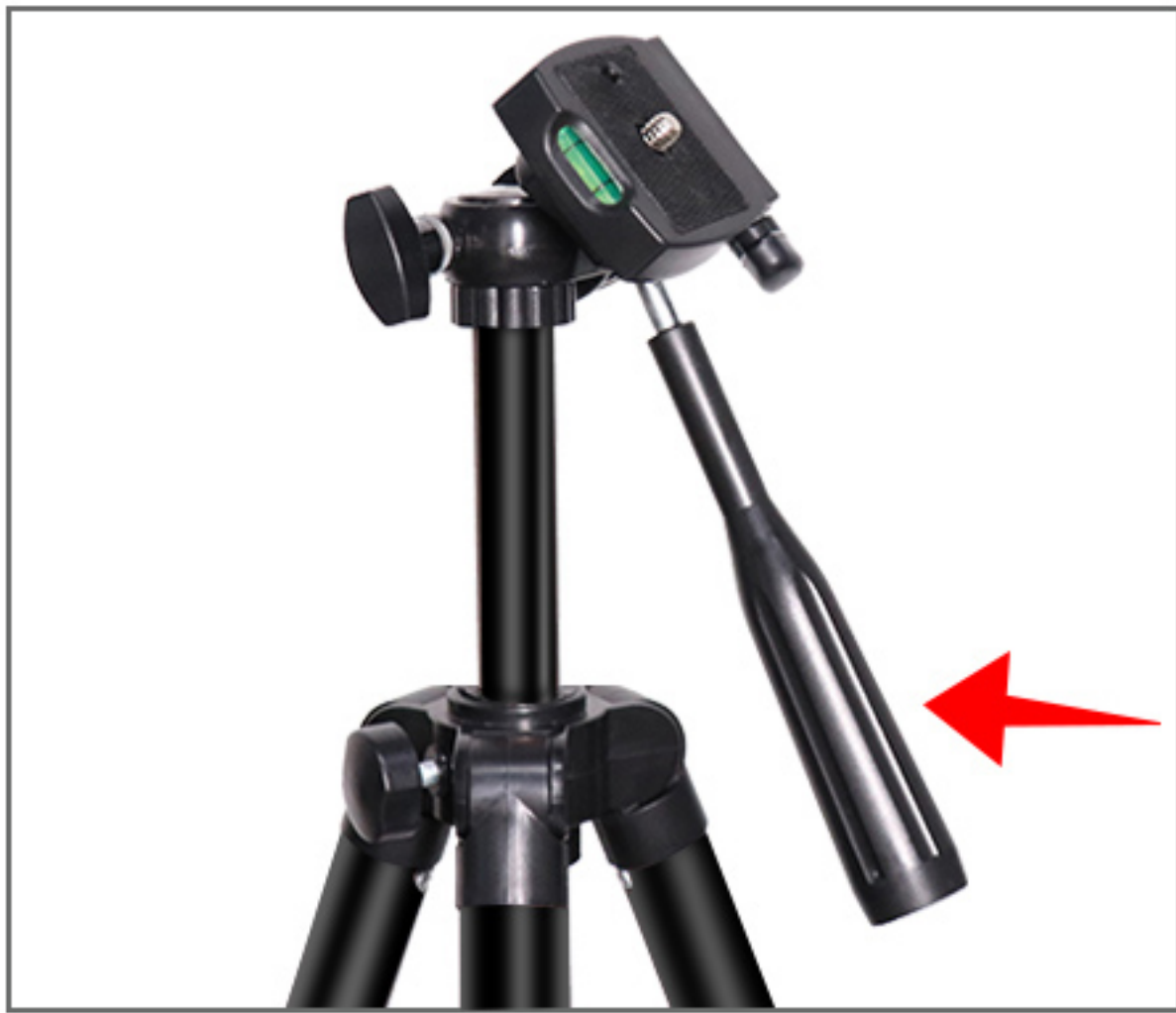
8. Vertical Shooting: Rotate the handle counter-clockwise and tilt the Pan head, allow maximum 90° for vertical use. Clockwise rotate the handle to lock.
