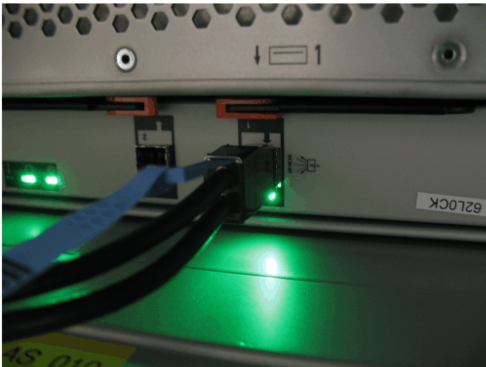
Figure 89. SAS cable correctly inserted into the SAS port
