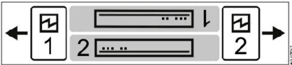
Figure 1. Label showing the orientation of the node canisters and PSUs
