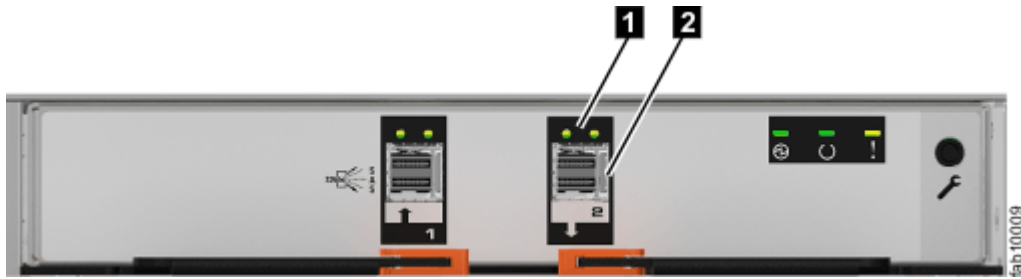
Figure 5. SAS ports and LEDs in rear view of an expansion canister for 2076-724
