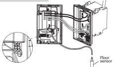
Reinstall the front part of the thermostat on the mounting base and tighten the screw at the bottom of the unit;
