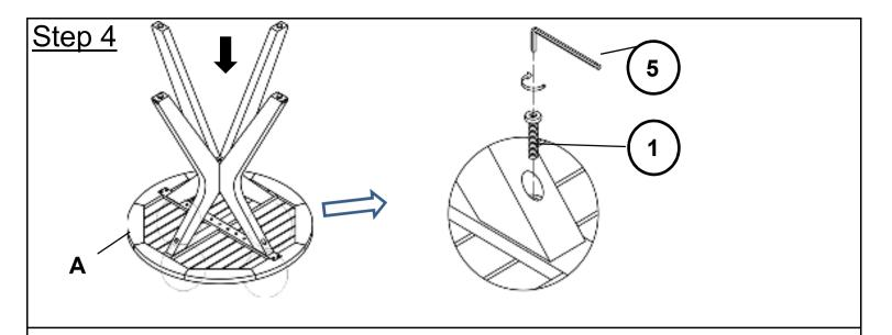
Attach Leg Frame to the Table Top(A) using Bolts( $\widehat{1}$ ) with Allen Key( $\widehat{5}$ ). **Do not fully tighten the Bolts**.
