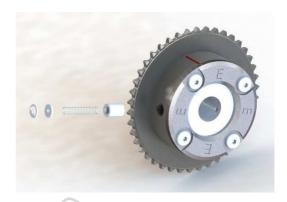
2. Using the ¼ inch drive Torx Bit supplied, remove the bots that hold the sprocket caps. Clean excess old engine oil off end caps and bolts, taking care not to damage the end cap working surfaces. Please note that sprocket "E" has smaller diameter caps and sprocket "A" has larger diameter caps. The bolts are all the same.
