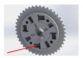
4. Carefully remove centre core of each sprocket and clean off excess old engine oil.
