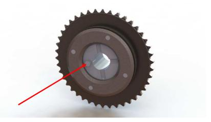
5. Carefully make sure that there is no excess grease in the holes or the threads. If there is, carefully wipe it out with some solvent and a cloth.
