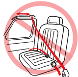
Lap Belt with Motorized Shoulder Belt
