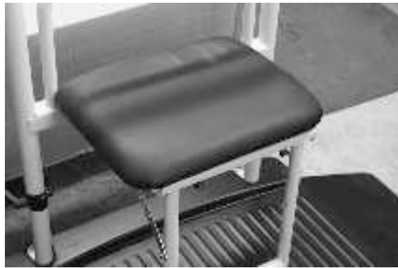
Figure 2-6. Chair Extended Down, Ready for Weighing Patients
