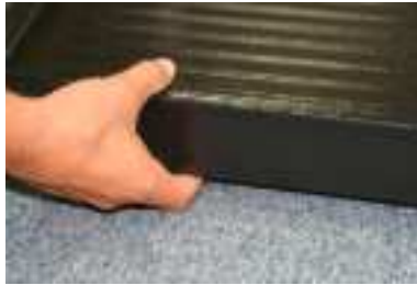
Figure 2-2. Clearance Between Scale Base and Floor
