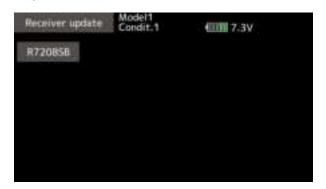
® The update screen is displayed. Connect the receiver or gyro to be updated to the S.I/F connector of the transmitter, prepare for update, and then tap the [Update] button.
