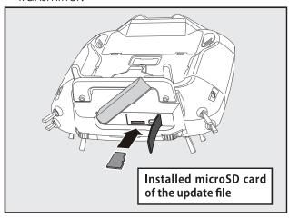
Turn on the transmitter power while pressing down the "HOME/EXIT" button. The update screen appears on the LCD display of your T16IZ SUPER and the software update is started.
