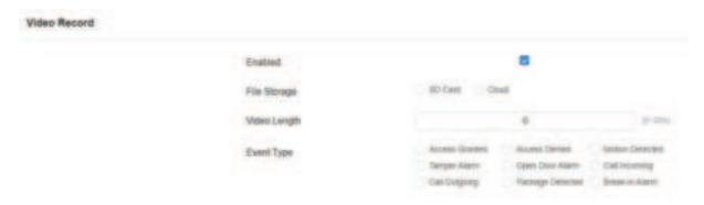
• File Storage: Store the videos in the SD Card or the SmartPlus Cloud. Only when the device has an SD card inserted or is connected to the SmartPlus Cloud will these two options display. When videos are stored in the SD card, the storage path is date/event/event details.
