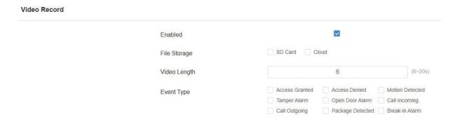
• File Storage: Store the videos in the SD Card or the SmartPlus Cloud. Only when the device has an SD card inserted or is connected to the SmartPlus Cloud will these two options display. When videos are stored in the SD card, the storage path is date/event/event details.
