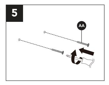
6. Leave 0.2 in. of the screws exposed. Hang the fixture (A) on the two screws (AA).
