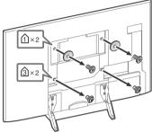
3 Attach the Wall-Mount Attachment (supplied with the TV) to the rear of the TV (to make it parallel with the wall). (XBR-65X930E only)
