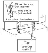
The length of the M4 machine screw differs depending on the rope or chain diameter. Please see below illustration.
