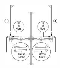
2. Install the upper side of bracket: Place  $\ensuremath{\mathfrak{D}}$  and 4 as shown, fix them with 4 sets of M6 \* 50 screws and nuts.
