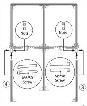
4. Install the lower side of bracket: Place (3) and 4 as shown, fix them with 4 sets of M6 \* 50 screws & nuts.
