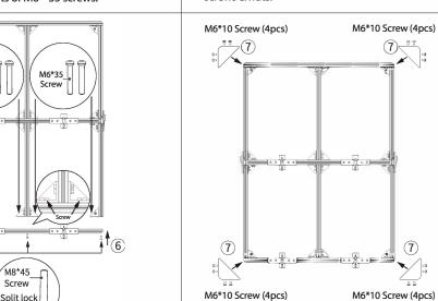
6. Install the corner guards of middle bracket: Place 7 as shown, fix them with 4 sets of 4 pieces M8 \* 45 screws.
