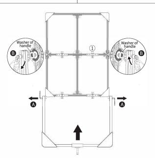
9. Combine the middle and bottom of bracket: Place the components installed in step 6 and step 8 as shown, pull the bottom bracket handle outward (Figure A), push the bottom bracket from bottom to top until the yoke rosettes are flush with the rosettes on both sides of the component ①, and tighten the left and right handles to secure the bracket onto the yoke (Figure B)
