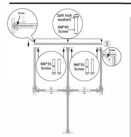
3. Install the upper of bracket: Place ⑤ as shown, fix it with 3 sets of M8 \* 45 screws & split lock washers and 8 sets of M6 \* 35 screws.
