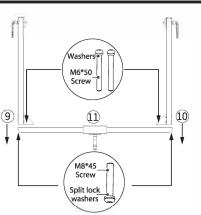
7. Install the bottom of bracket: Place (9 (11) (11) as shown, fix them with 4 sets of M6 \* 50 screws & washers and 2 sets of M8 \* 45 screws & split lock washers.
