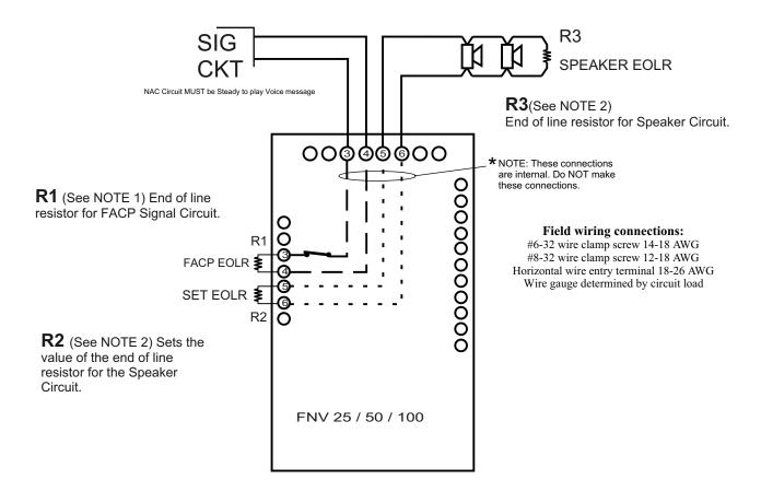
**NOTE 1**: If the Fire Alarm Signal Circuit requires a 4.7K end-of-line resistor, then R1 must be a 4.7K. Normally, this resistor is connected to the Signal Circuit through a closed Trouble contact. When the FNV 25/50/100 goes into Trouble, the contact opens, producing an "Open" on that Signal Circuit, notifying the FACP.
