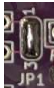
Bad Solder Bridge All pads connected
