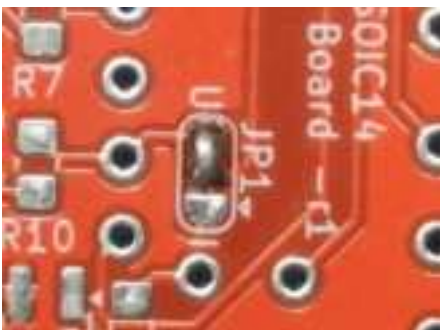
Solder jumper selecting UPDI programming option
