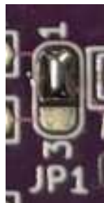
Step 2 Completed Bridge
