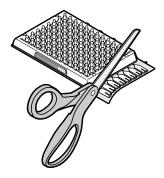
**IMPORTANT!** Completely remove the fill reservoir strip. Any remaining plastic that extends beyond the card edge can prevent the card from seating properly on the sample block and can affect amplification.
