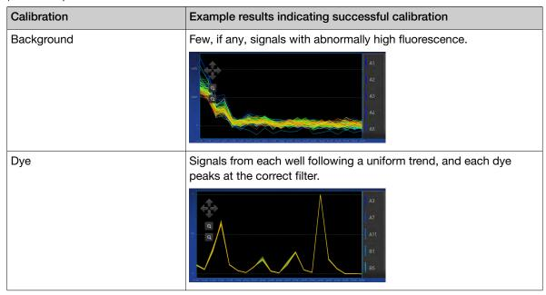
5. *(Optional)* For Uniformity, Background, and Dye calibration images, tap on an individual well on the right side to see the results for a single well.
