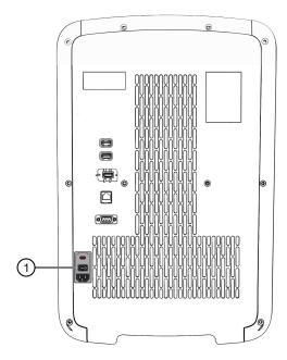
Figure 24 Location of the ON/OFF switch
