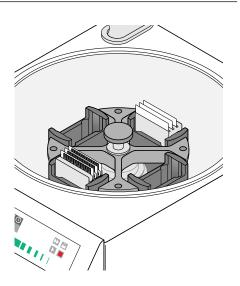
Centrifuge is properly loaded and balanced.
