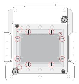
The circles indicate the guides for the position of the array card.
