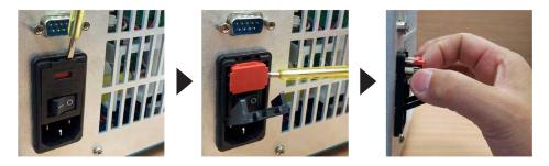
Remove each fuse from its fuse holder, then inspect it for damage.
