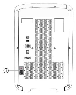
Figure 6 Location of the ON/OFF switch
