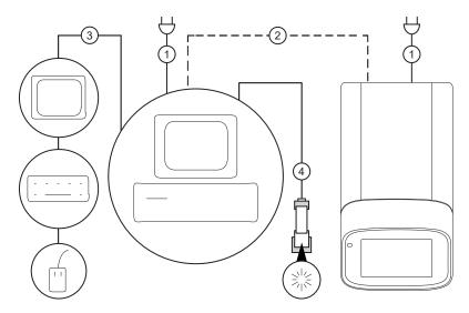
Figure 26 Instrument-to-computer connections (minitower configuration)
