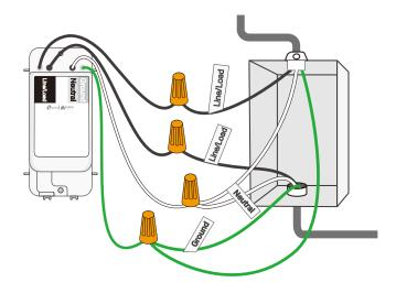
Note: No need to distinguish between Line and Load wires.
