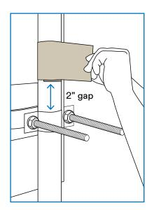
Adhere one end of the absorber stripe to the pole and wrap the absorber around the surface.
