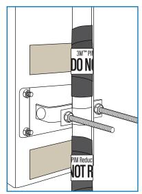
Remove absorber liner and apply above and below bracket attachment location, allow 2" gap.
