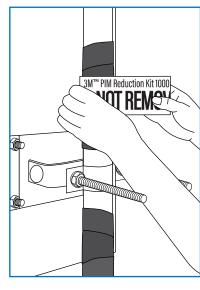
Apply "Do Not Remove" label around the previously installed tapes and place additional labels as desired.
