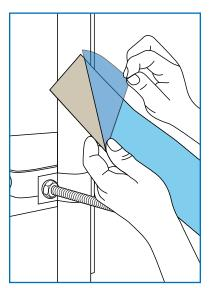
Expose adhesive surface by removing liner for the 3M™ External PIM Absorber 1000.
