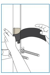
Wrap the tape with ½" overlap and use minimal tension.
