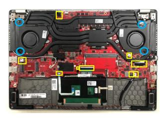
Remove module (MB+Thermal+FAN)
