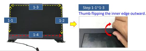
Due to some tapes behind the lower edge of bezel, please using plastic blade to teardown the bezel.
