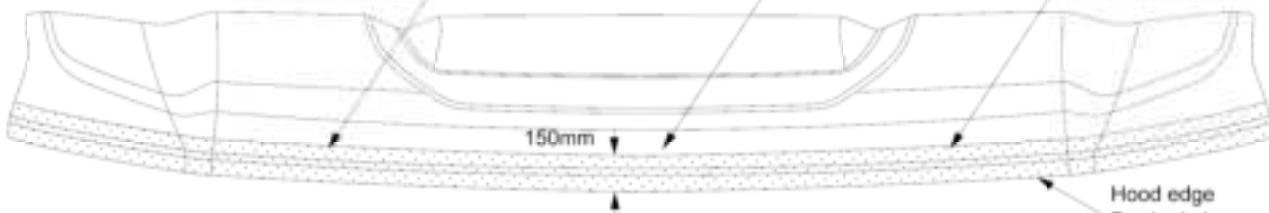
Using one of the surface wipes **B** provided and clean the first 150mm of front of the hood.
