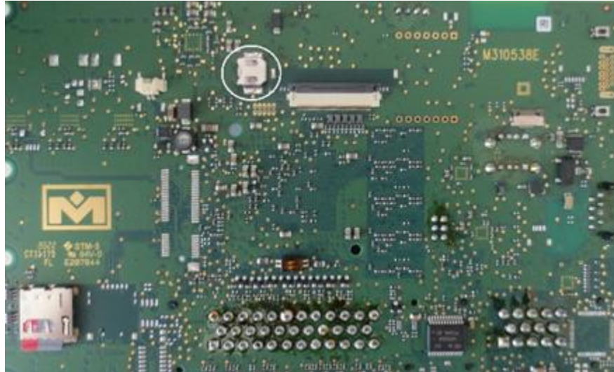
Figure 3: Localisation of the battery (white circle) on the PCB of the MConn 7.
