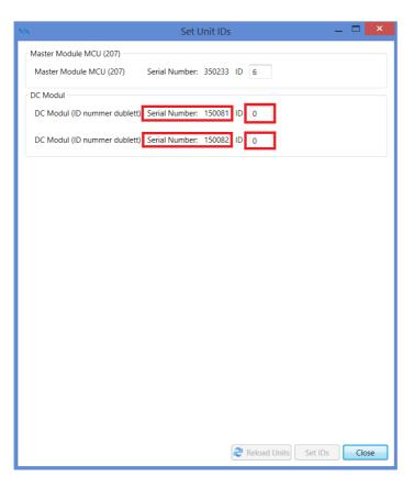
**3.6** Input the ID number that correspond with the module in the I/O list and the Set ID's. **Note**: You can always change the ID's in the project explorer/properties.
