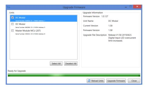
**3.4** The program will notify if a upgrade is necessary by having filled in the checkboxes automatically. Choose Upgrade firmware if needed.
