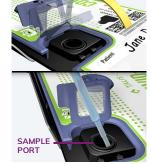
8 Dispose of pipette and close lid until it clicks, then cap sample tube.
