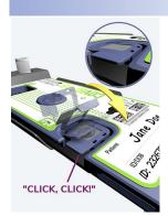
**Q** Insert Cartridge until it clicks, with label facing right. Instrument begins reading the Cartridge.
