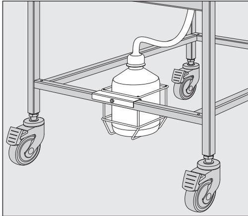
It is possible to attach a holder for the drip bottle (accessory sold separately) to the strut under the drain connection.
