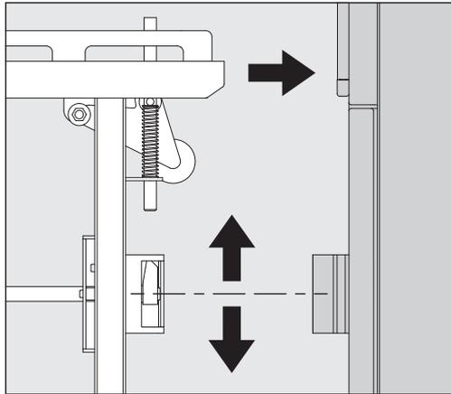
The height of the transfer trolley can be adjusted at the wheels. The height must be set so that the docking mechanisms of the transfer trolley and the machine engage.
