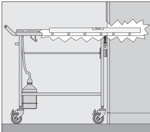
The conveyor rollers on the transfer trolley and in the machine must be at the same height so that the load carrier can be moved easily.
