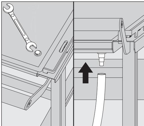
A drain connection is located on the right-hand side of the drip tray. There is a blind stopper closing off the drain connection when the equipment is in its as-delivered state.
