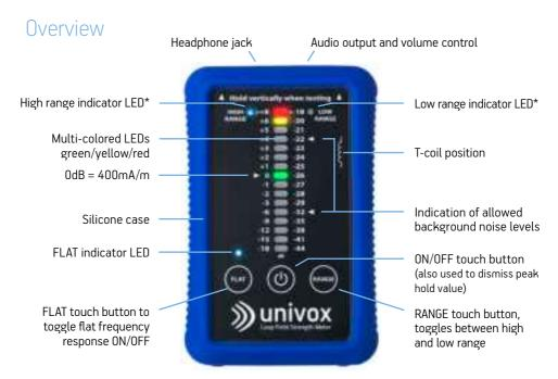
\*The range indicator LEDs flash blue when the battery is low
