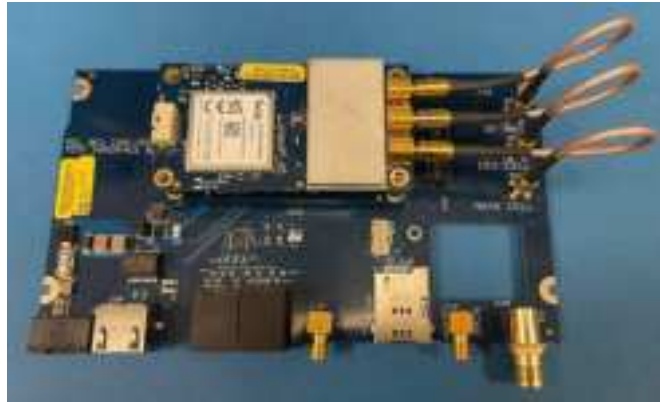
Figure 8: OCR220 Module Installed on test fixture
