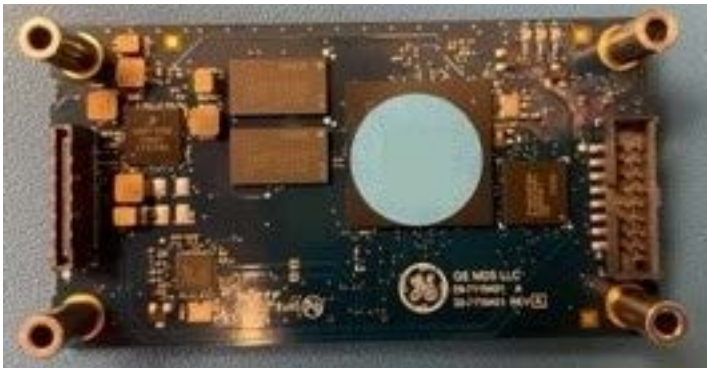
Figure 3: OCR220 Processor PCBA
