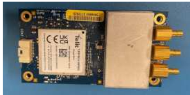
Figure 2: OCR220 Radio PCBA
