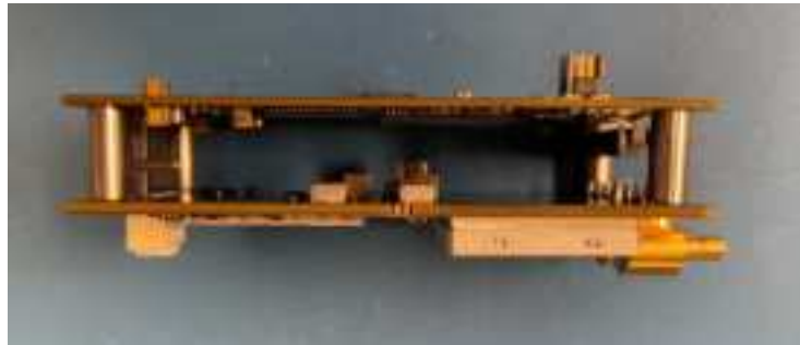
Figure 1: OCR220 Module. Bottom PCB is radio (Figure 2) and Top PCB is processor (Figure 3)
