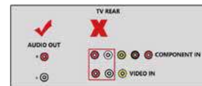
Fig 3-7 Use the right RCA ports
