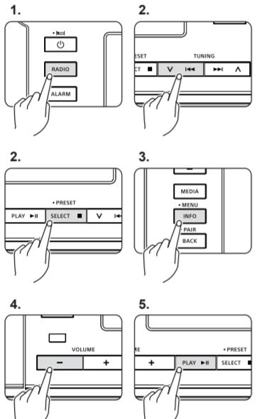
2. Navigate the radio's on-display menu's by using the V / < > / ▲ and SELECT / ■ buttons to find the Internet radio station or Podcast that you want to listen to.
