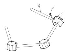
Attach a new hexagon for three rods (1) to the latest rod. Fasten with a screw (a). Keep in mind both the rotation of the holes and that the engraved mark should be facing outwards. See Pic. 6.
