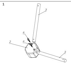
Assemble the bottom hexagon: Take one of the hexagons for 2 rods (2) and install two rods (3). Rotate the rod so that the angle of the hole in it lines up with the angle of the screw-hole in the hexagon. Join the pieces with a screw (a) using the hex key (b). See Pic. 1.
