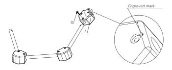
Next attach a hexagon for 3 rods (1) to the new rod. Fasten with a screw (a). Rotate the new hexagon so that the engraved mark is facing outwards. See Pic. 4.
