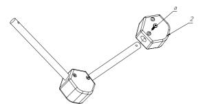
Attach a hexagon for 2 rods (2) on one of the installed rods. Fasten it with a screw (a). Mind that the overall angle should be inward. See Pic. 2.
